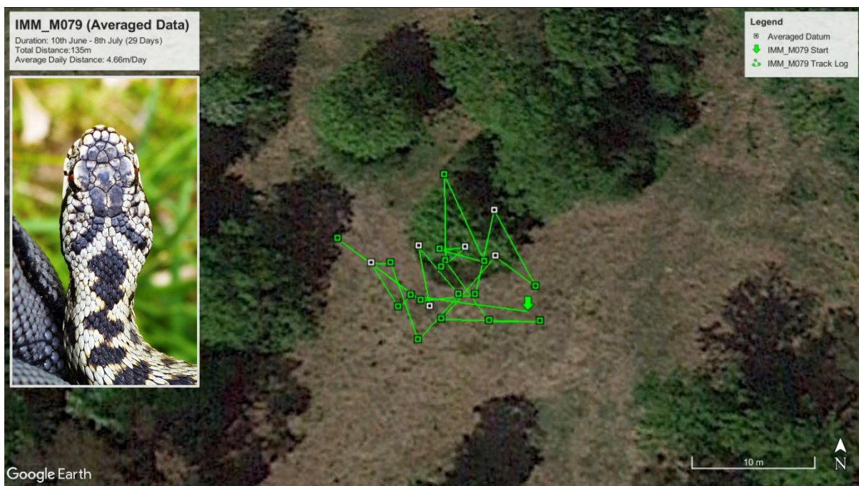
Figure 38. Track log for IMM_M079. White icons represent points that have been averaged. At such a small scale, the error in GPS accuracy becomes more apparent. GPS points have been averaged for consecutive records at the exact same location (determined from field notes).
